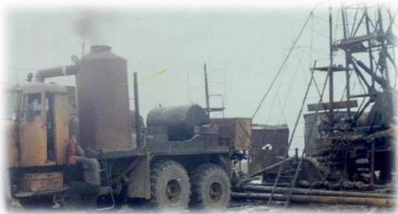
Hot Diesel Application
